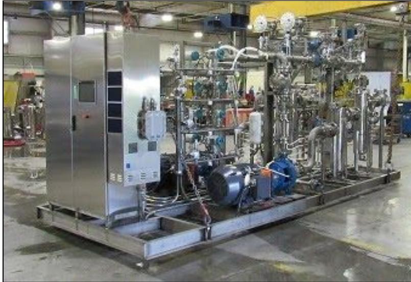
PRM constructed multiple custom stainless steel washing skids. Each was built on an open 304SS skid. The systems were integrated into a Siemens HMI PLC control platform to allow the operator complete control of the washing cycles. All components on each skid were either 304SS or 316SS and wired for Class 1 Div 2 hazardous locations.
