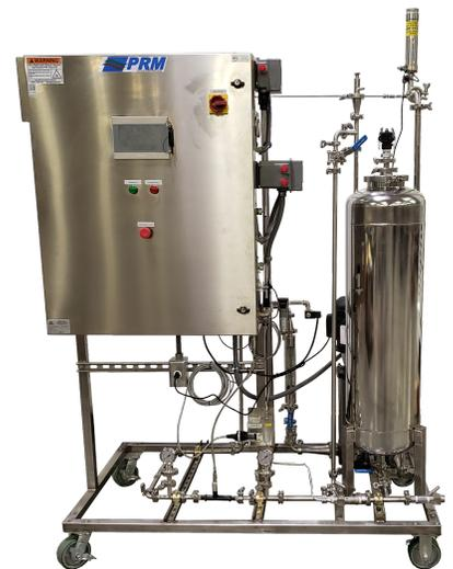
Ozone oxidation is one of the most effective water treatment processes, and is very environmentally friendly since it is produced onsite from oxygen and reverts back to oxygen after reacting with contaminants.
