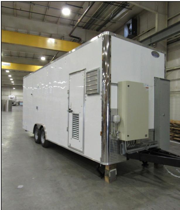
This multi-phase extraction and air sparging system was packaged in an 8' x 26' dual axle cargo trailer. The system included a MS-400 moisture separator and 200 gallon water storage tank. A PRM model STS-334 sliding tray air stripper was situated in the rear of the trailer. The system also included two PRM model HP-500 carbon vessels. The PLC was mounted to the exterior of the trailer to allow more room in the interior.
